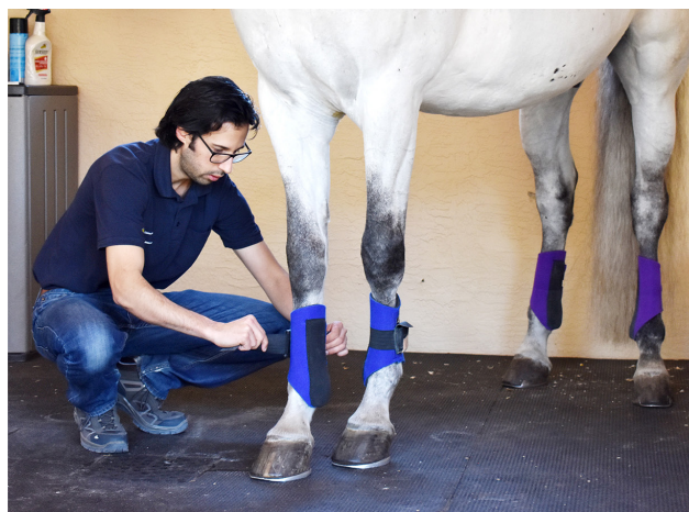
FIGURE 1. The EquiMoves system uses small inertial sensors that attach to the horse using adhesive pads. At left, Dr. Elin Hernlund centers a sensor over a horse's pelvis. At right, Dr. Filipe Bragança puts on brushing boots containing pockets for sensors that will measure movements of the cannon bones.
