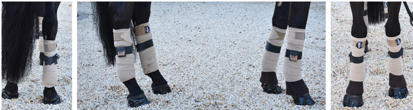
FIGURE 2. Sensors attached to all four limbs. Sensors on the cannon bones are securely attached in brushing boots. Hoof sensors are taped directly onto the hooves, then covered with tape for extra protection.
